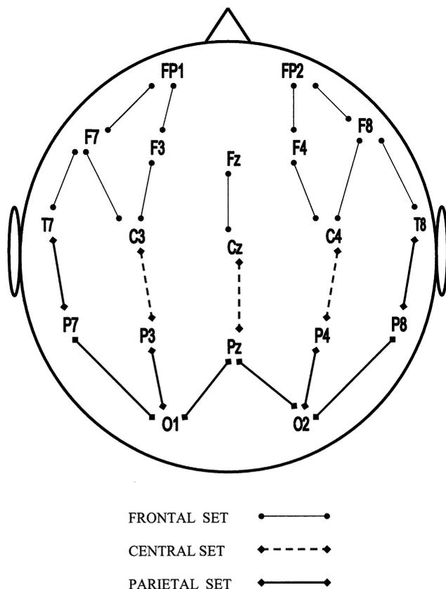
Figure 1. Topographical diagram of the electrode-pairs.
